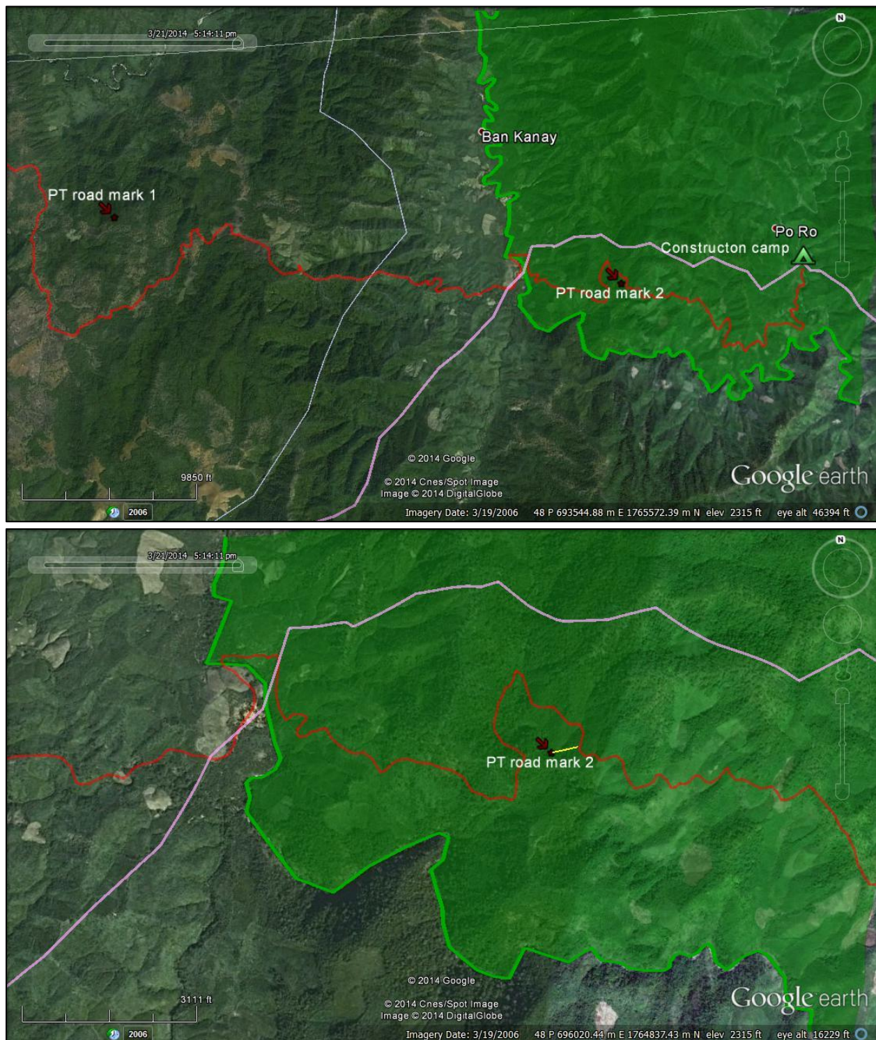
Figure 28. Comparison of the constructed road (highlighted in red) with the variant on the first scheme (light purple) and geo-referenced points taken from the second scheme.
